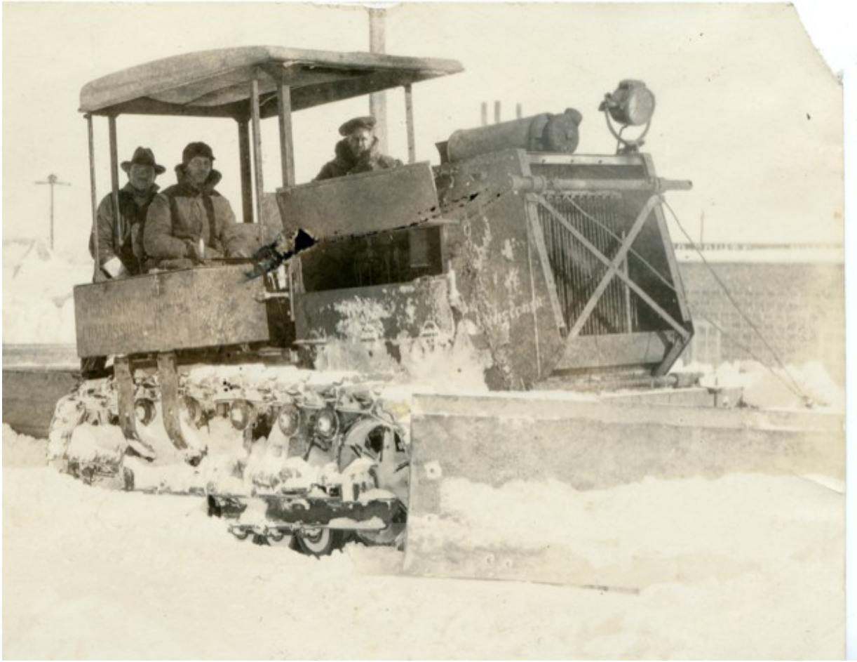
Price County's Holt Ten Ton Caterpillar Tractor used for snowplow work on county and town roads. This Cat was used on the morning of Friday, February 24, 1922 to clear the roadway through Phillips during the Great Snow and Ice Storm that hit the entire State of Wisconsin. Price County Historical Society, Inc. Archives Collection.
